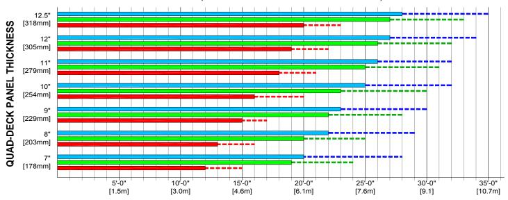
**CLEAR SPAN** (Center to Center of Load Bearing Support)
